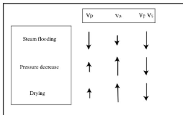
**Figure 2: The effects of processes caused by exploitation at The Geysers on  $V_p$ ,  $V_s$  and  $V_p/V_s$ . Large arrows indicate the dominant effect and small arrows indicate subsidiary effects. The three processes have differing effects on  $V_p$  and  $V_s$  but all cause  $V_p/V_s$  to decrease.**
