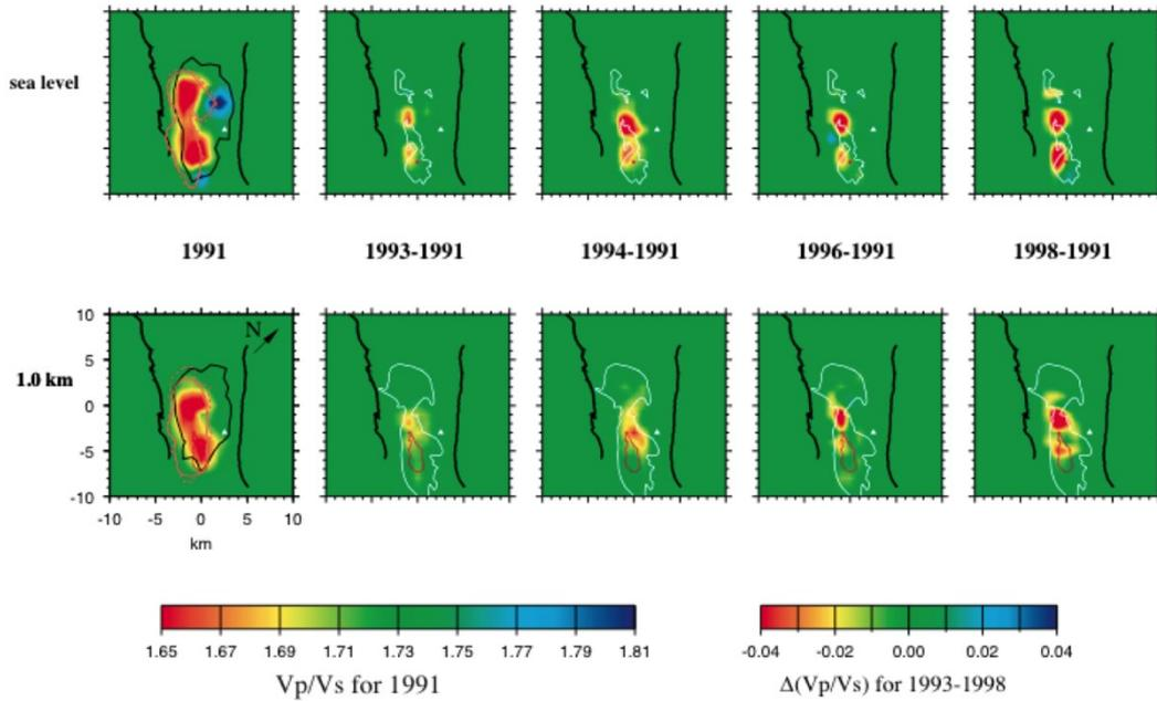
**Figure 1: Maps showing changes in the  $V_p/V_s$  ratio at two depths at The Geysers geothermal area, California, between 1991 and 1998, as determined by Gunasekera et al. (2003) by inverting five data sets independently.**
