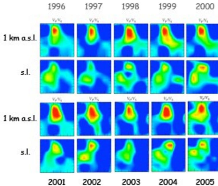
**Figure 8: A selection of results from independent tomographic inversions of the Coso geothermal area, California. Top two rows of panels:  $V_p/V_s$  for horizontal slices at 1 km above sea level and at sea level, for the years 1996 - 2000. Bottom two rows of panels: same as top two rows except for the years 2001 - 2005.**
