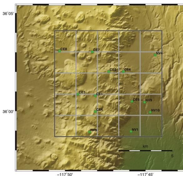
**Figure 3: Map of the Coso geothermal area, eastern California, that we used as the basis for synthetic tests. Green squares: Stations of the U. S. Navy’s telemetered seismometer network. The tomographic grid has nodes spaced by 2 km horizontally and 1 km vertically.**
