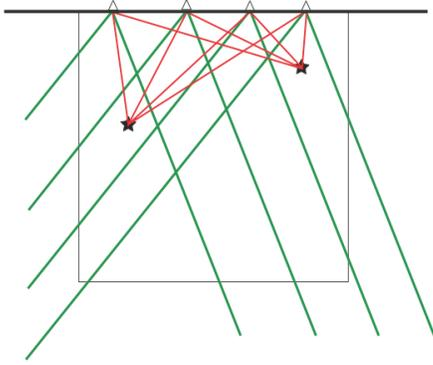
Figure 1: Schematic diagram of seismic ray coverage from different kinds of earthquakes. Heavy horizontal line: Earth's surface; Triangles: Seismometers; Square: volume of interest such as a geothermal area; Stars: Local earthquakes. Rays from local earthquakes (red lines) provide no coverage below the seismically active volume (and require local seismicity). Rays from more distant (regional) earthquakes (green lines) sample the entire volume of interest, even in the absence of local seismicity.
